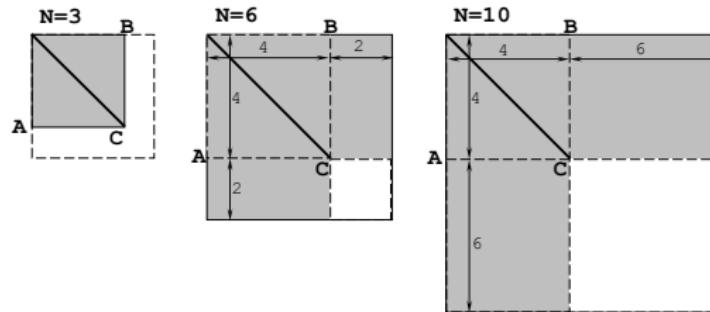
**Configuration of GEMM update:**  $C_{m \times n} = C_{m \times n} - A_{m \times k} \times B_{k \times n}$
