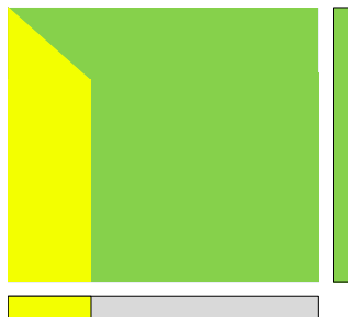
Fig. 6. Separation of lower and upper areas protected by checksum (green) and checkpoint (yellow) during the course of the factorization algorithm
