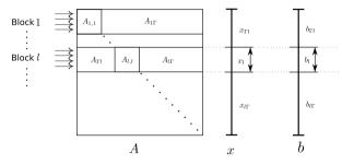
**Fig. 2.** Visualizing the asynchronous iteration in block description used for the GPU implementation.
