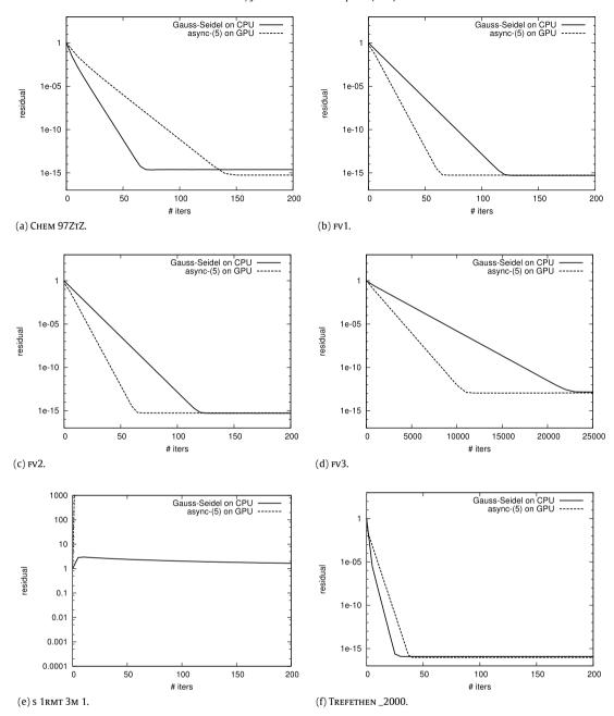
Fig. 7. Convergence rate of block-asynchronous iteration.
