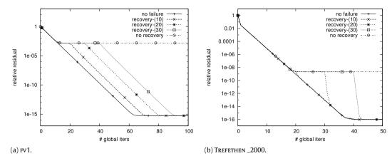
**Fig. 10.** Convergence of async-(5) for hardware failure. The implementations either recover by reassigning the components to other cores after the recovery time  $t_r$  (denoted by recover- $(t_r)$ ), or generate a solution approximation with a significant residual error.
