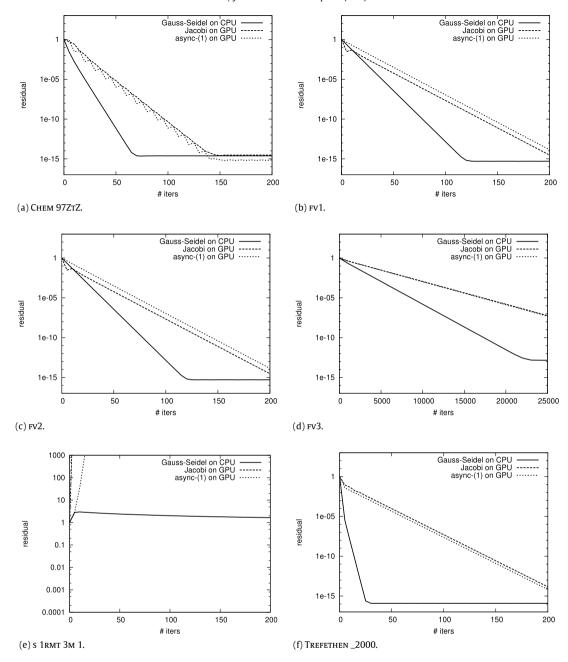
Fig. 6. Convergence behavior for different test matrices.
