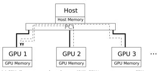
(c) GPU-direct memory kernel access (DK), GPU1 serves as master-GPU.
