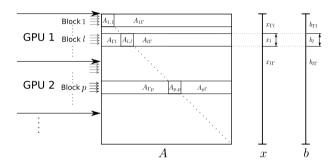
$\textbf{Fig. 3.} \quad \text{Visualizing the block-asynchronous iteration for multi-GPU implementation.}$
