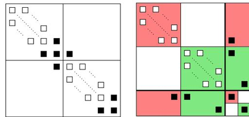
(a) Original tridiagonal matrix. (b) Matrix after reordering.
