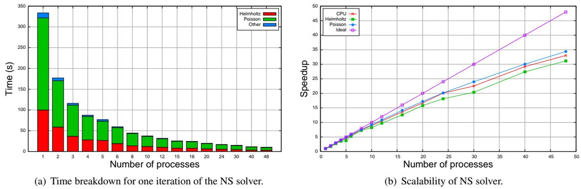
Fig. 7. Performance of the Navier-Stokes solver.
