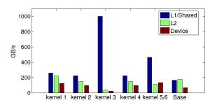
Figure 7: Memory bandwidth of previous(base) and optimized kernels. The theoretical peak bandwidth of device memory of K20 is 208GB/s.
