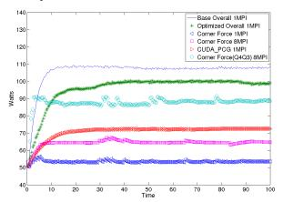
Figure 15: One K20 power. Except denoted, all are with a  $Q_2$ - $Q_1$  method.
