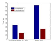
Figure 3: Performance of kernel 1,2 with local memory and register arrays, respectively. Test is performed on K20 for a 3D  $Q_2$ - $Q_1$  case.
