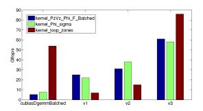
Figure 6: The performance of kernel 3,4,7 on K20. v1 is the straightforward implementation. v3 is the optimized and tuned result.
