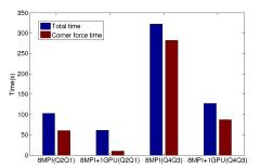
Figure 11: Speedup of CPU-GPU code over the CPU. A 1.9x overall speedup is obtained on  $Q_2$ - $Q_1$ ; 2.5x on  $Q_4$ - $Q_3$ .
