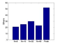
Figure 4: Tuning of kernel 3 which achieved 60% of theoretical peak performance on K20. N is the number of matrices performed in each thread block. The optimal N is found by auto tuning.
