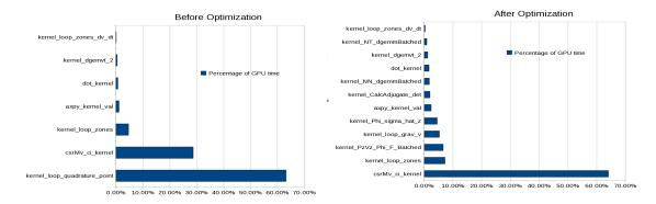
Figure 5: Kernel time distribution of the base versus redesigned and optimized implementation
