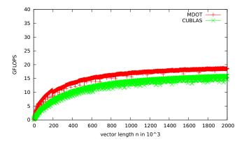
Fig. 9. Performance comparison between CUBLAS and MDOT for the sequence of dot products in one BiCGSTAB iteration.
