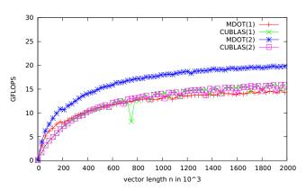
Fig. 8. Performance comparison (double precision) between CUBLAS and MDOT executing 1 and 2 vector products.
