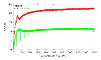
Fig. 5. Performance comparison between the merged BiCGSTAB and the reference implementation for the update of vector p (see line 11 of Figure 1).
