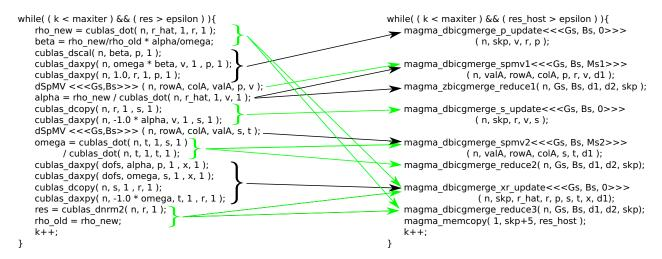
Fig. 3. Visualizing the reformulation of the reference BiCGSTAB implementation (left) to the optimized version (right). While all parameters remain in GPU memory, note the explicit transfer of the residual back to the host in the last line.
