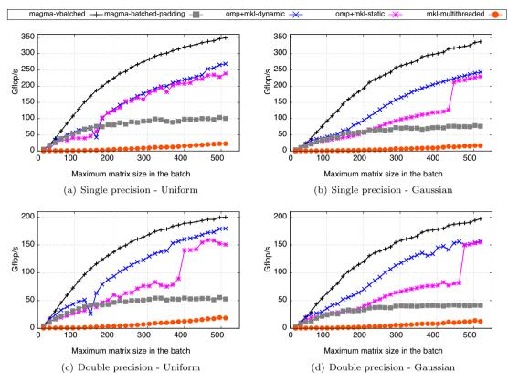
Figure 6: Performance on batches of variable sizes, batchCount = 3,000.
