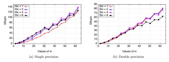
Figure 3: Impact of tbc on performance, batchCount = 10,000, on a K40c GPU.
