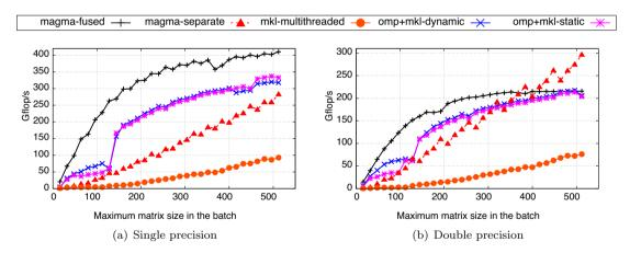
Figure 5: Performance on batches of fixed size, batchCount = 3,000.
