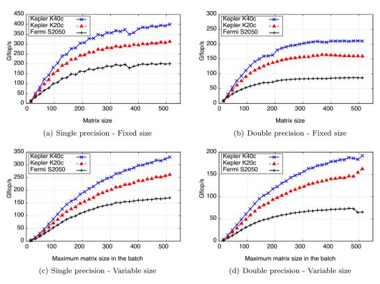
Figure 7: Performance on different GPUs, batchCount = 1,000.
