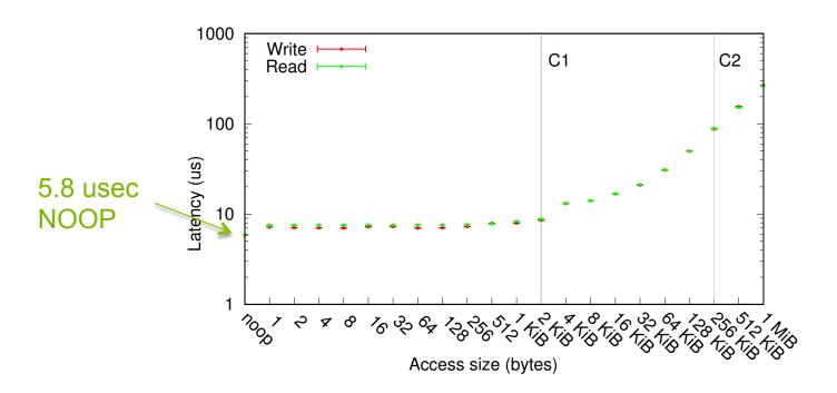
FDR IB, RAM disk, 2.6 usec round-trip (MPI) latency measured separately
