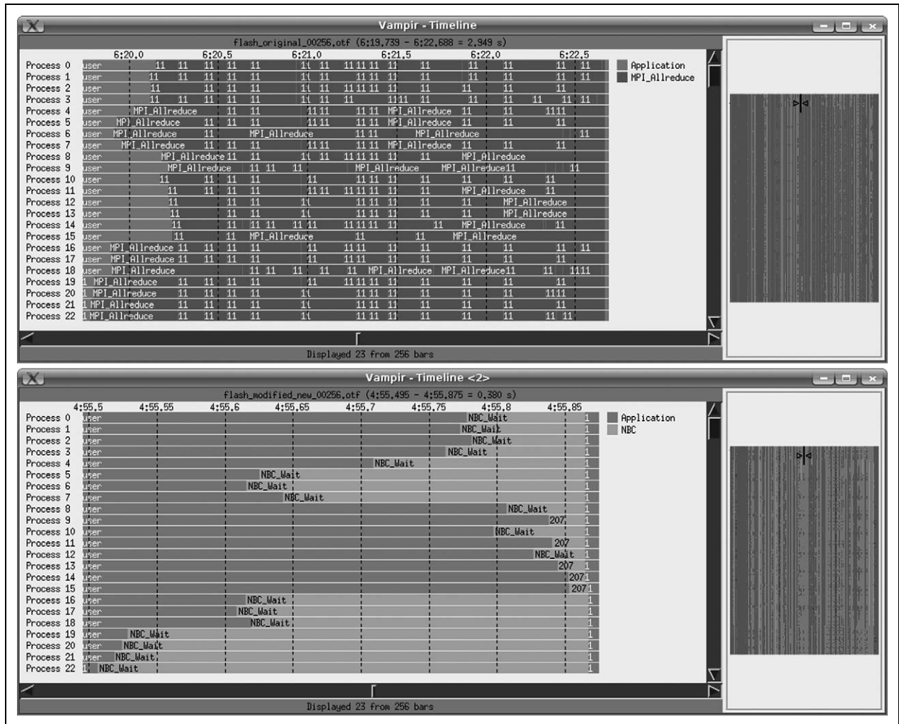
Figure 2. Corresponding communication patterns of MPI_Allreduce in the original code (top) and NBC_iallreduce plus NBC_Wait in the optimized version (bottom). The latter is more than seven times faster, taking 0.38 s instead of 2.95.
